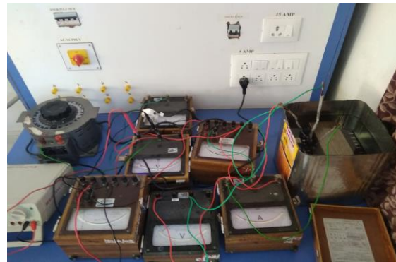
Figure 3: Photograph of oil cooling experimental setup.
